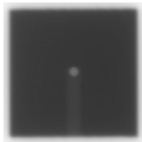
FIG. 1. One example of eight original images of the reference ball-bearing used in the Elekta XVI software.
